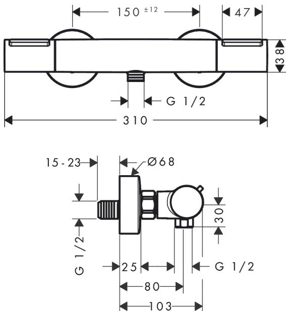
**Ecostat Element****Brausethermostat Aufputz**Oberfläche: **Chrom** Artikelnummer: **13346000**
