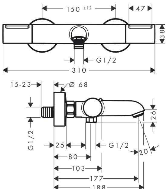
**Ecostat Element****Wannenthermostat Aufputz**Oberfläche: **Chrom** Artikelnummer: **13347000**
